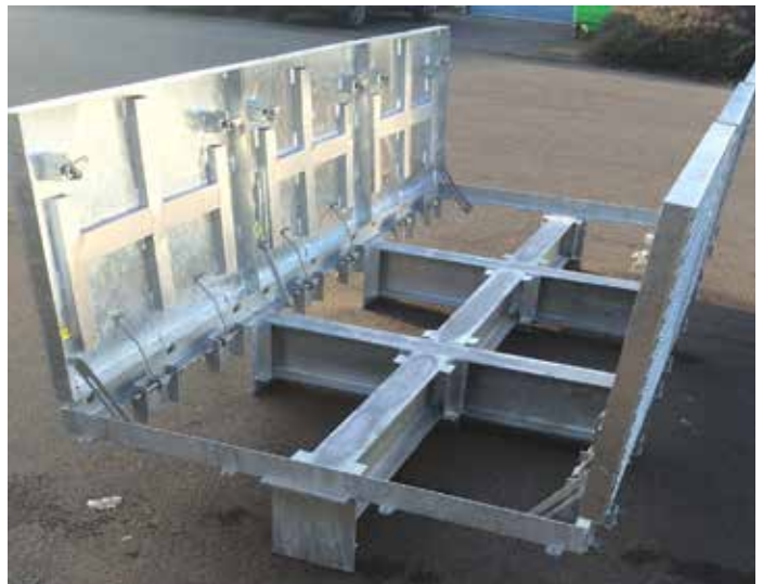
New cover & frame awaiting dispatch
